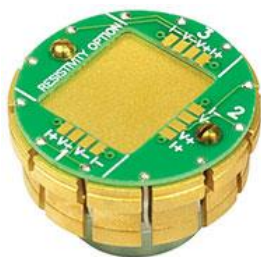
Figure 2.16: Standard three channel pucker for PPMS measurements
