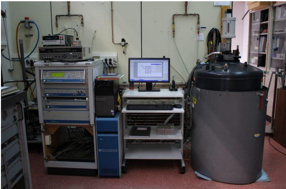
Figure 2.15: Image of the PPMS located in the ICMM (CSIC). The helium chamber is on the right and the electronics are in the left of the image.
